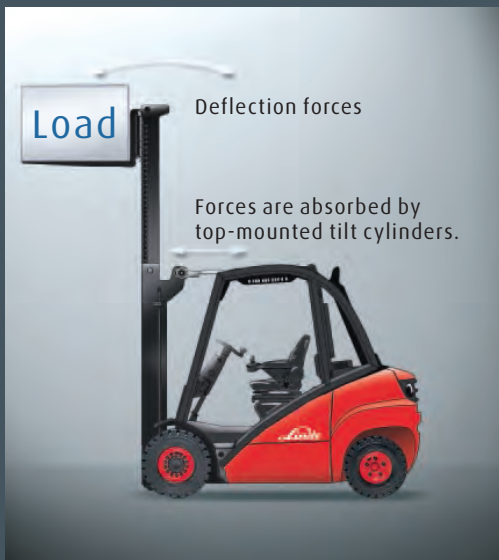
Clear-visibility mast. Top-mounted tilt cylinders allow use of narrow mast sections.
